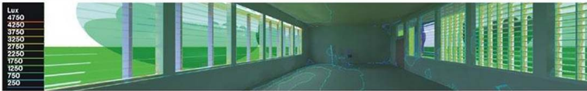
INTERNAL PANORAMIC VIEW – DECEMBER, 21st, 12:00 PM, ILLUMINANCE LEVEL, CIE CLEAR SKY & SUN
