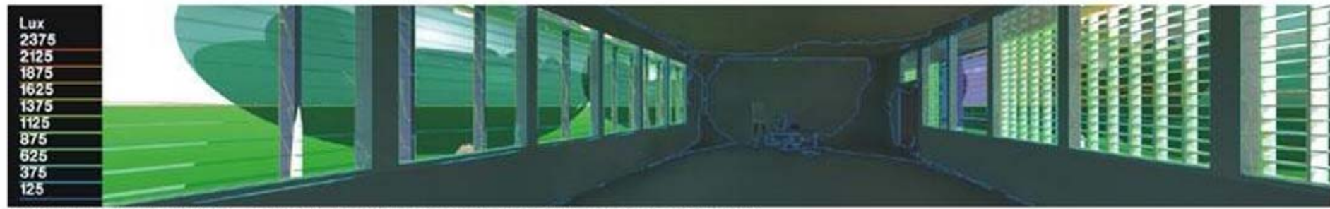
INTERNAL PANORAMIC VIEW – JUNE, 21st, 8:00 AM, ILLUMINANCE LEVEL, CIE CLEAR SKY & SUN
